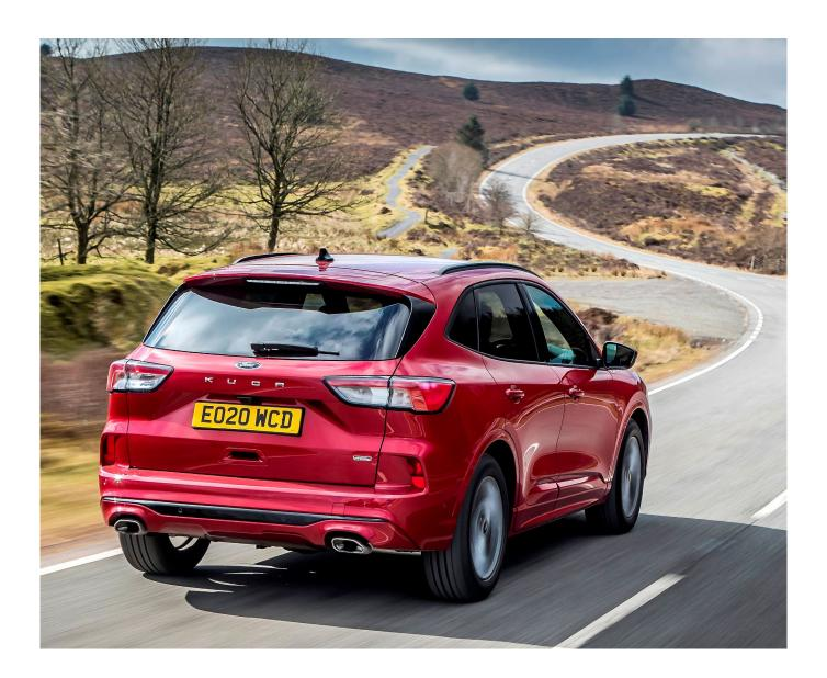
On the technical aspects the Kuga PHEV uses a 2.5 litre, four cylinder Atkinson-cycle, DOHC petrol engine with variable cam timing combined with an electric motor and generator with a 14.4kWh lithium-ion battery. The total power output is 225 hp with drive to the front wheels through a CVT single forward speed plus reverse auto transmission. Top speed is 125 mph and zero to 62 mph takes 9.2 seconds.
