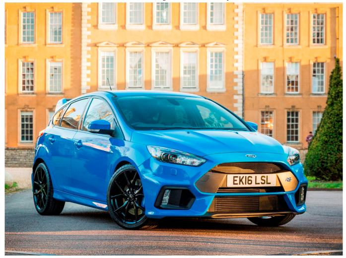
There are four performance driving modes – Normal or Sport for on-road driving and Track or Drift modes for track use. The car also has launch control and sports suspension with stiffer spring rates increased by 33% at the front and 38% at the rear, plus more efficient roll bars over those used for the Focus ST. The suspension has two modes, Normal and Sport, the latter being 40% firmer for track driving. A linear input electric power steering
