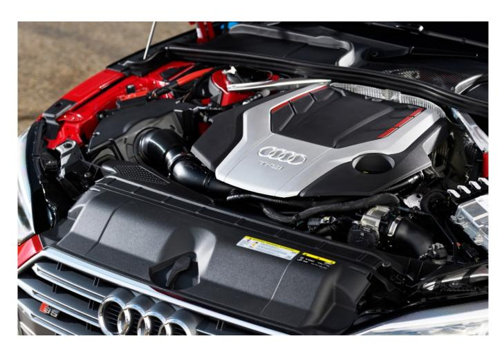
At the heart of the latest S5 is a new 3.0 litre, V6, TFSI direct injection petrol engine which replaces the old 3.0 litre, supercharged 333 hp V6 unit, with the new engine being the basis for the forthcoming RS road versions and DTM touring car machine. In this road going form it provides 354 hp from 5,400 rpm but also a massive 500 Nm (369 lb.ft) of torque is developed from only 1,370 rpm. This power is 6.5% more than the old engine, with 13.5%
