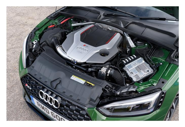
Perhaps the new 2.9 litre V6 twin-turbo direct injection petrol engine doesn't have the same 'theatre of noise' or acceleration exhaust howl of the old V8 which will be missed by petrolheads but we all should enjoy the endless supply of 600 Nm (442.5 lb.ft) of torque this new unit supplies over such a wide engine speed range from 1,900 to 5,000 rpm. The power
