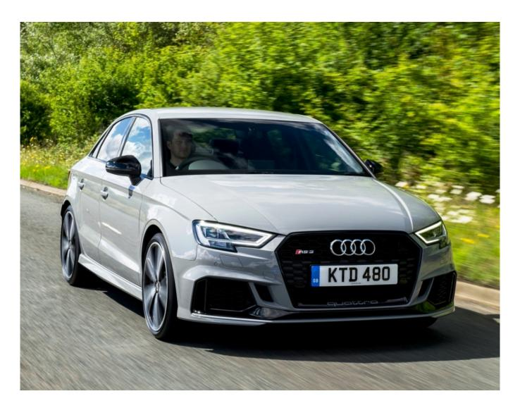
The first Audi RS 3 in Sportback form was launched in 2011 with a 335 bhp turbo petrol engine and four years later this power output went up to 362 bhp. Now Audi has pushed that power output up to 395 bhp or as we now call it 400 hp. It supplies a huge 480 Nm (354 lb.ft) of torque from 1,700 rpm right through to 5,850 rpm, and the driver can adjust – through the Drive Select function – the gear shift points and the proportion of torque directed to the rear wheels – which can be up to 100%.
