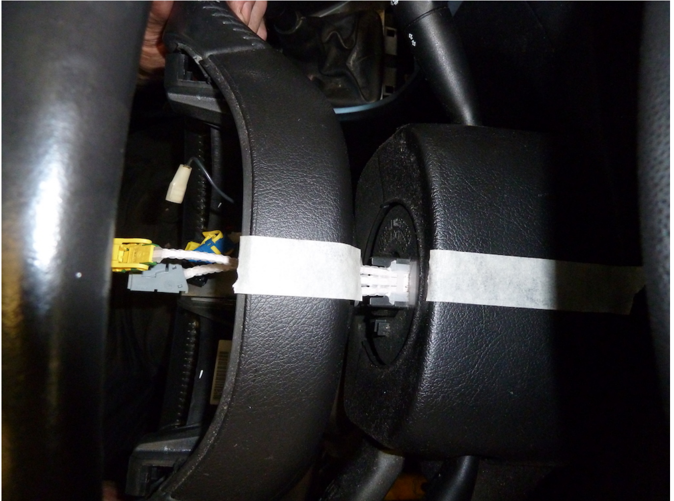
Masking tape can be used to mark the position of the steering wheel, prior to removal.
