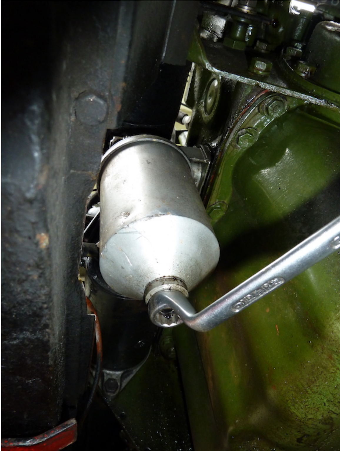
On many classics the engine oil filter element is located within a steel
