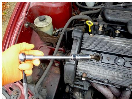
Use a quality spark plug spanner with a rubber insert that firmly grips the plug; essential when they live in deep wells...
