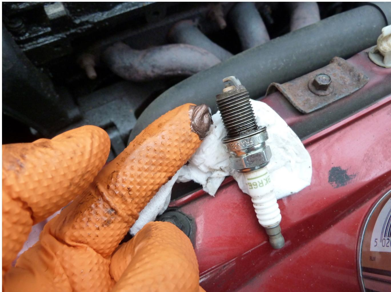
The application of a little copper-based anti-seize grease on re-installation will help prevent the plugs from seizing, aiding removal in the future.
