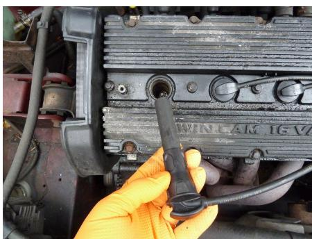
Take great care when detaching the high tension connector and lead from each spark plug; a special tool may be needed.
