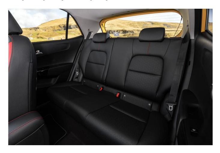
An offset split back-rest meant the luggage area could be gradually increased in capacity from taking just some bags of shopping or two medium suitcases to much bigger items under the fifth door with its sensible deep and long loadbed.
