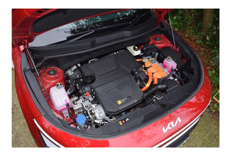
The powertrain drives the front wheels via Kia's second generation six speed dual clutch (DCT) automatic transmission. Interestingly, changes for this transmission include the use of low friction ball bearings, gears optimised for efficiency, and notably the removal of the reverse gear (this move alone saves 2.3 kg or 5.1 lb in weight). Reversing is now accomplished by using the car's electric motor, thus saving tailpipe emissions.
