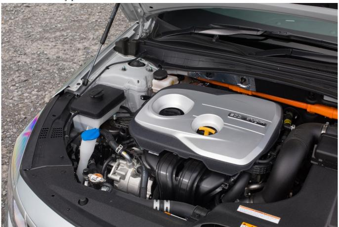
The Optima Sportswagon PHEV combines a 154 bhp 2.0 litre direct-injection petrol engine with a 50 kW (67 bhp) electric motor powered by an 11.26 kWh lithium-ion polymer battery pack. The electric motor replaces the torque converter in the six-speed automatic transmission. When working together, the combustion engine and electric motor generate 202 bhp and 375 Nm (277 lb.ft) of torque. Top speed is 119 mph and zero to 60 mph takes 9.4 seconds.
