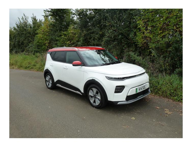
From the petrol-powered Picanto I stepped into the 'pure electric' Soul EV 'Explore', this distinctive SUV being driven by a permanent magnet synchronous electric motor, linked to a 64 KWh Li-on polymer battery. Power output is 64KWh or 202 bhp ('Urban' versions are rated at 39.2 KWh or 134 bhp).
