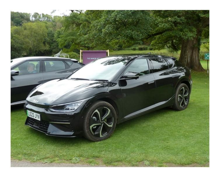
More pure electric motoring for me during my next drive, in the multi-award-winning EV6. My test car on this occasion was the GT-Line S' 77.4 kWh AWD version, delivering 321 bhp plus 605 Nm (446 lb.ft) torque from its twin motors. Power is fed to the tarmac via a single speed automatic transmission plus all wheel drive system.
