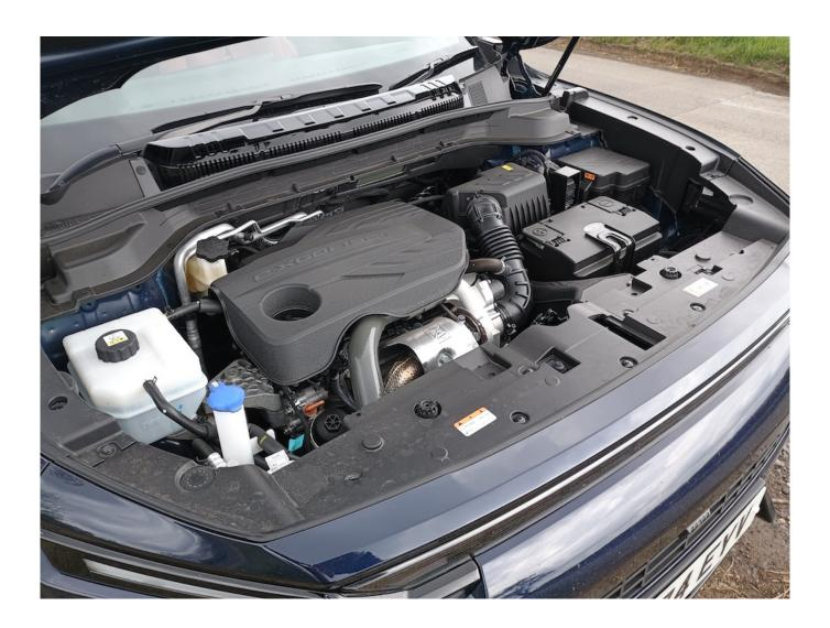
The engine incorporates an integrated exhaust manifold for more rapid warm-up from cold, an electro-magnetic circulation valve and an electronic carbon emission gate. 'Idle Stop and Go' (ISG) technology is also built in to save fuel and emissions.
