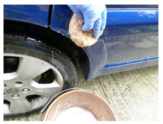
When washing a car, leave the lower parts of the vehicle until after tackling its upper sections. This will minimise the chances of scratching the glass and the paint, due to grit on the sponge.
