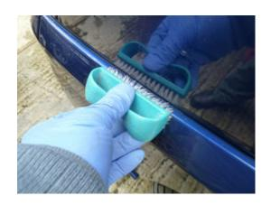
For harmlessly removing stubborn deposits from the paintwork, and from around the window seals, the gentle application of an old, soft-bristled brush is effective.
