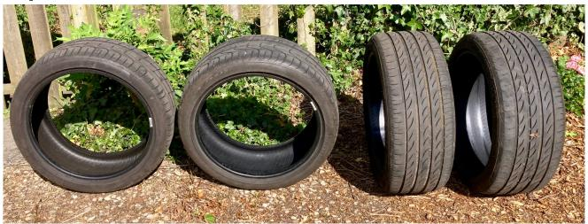
Reason? After exhaustive—and free—pre-fitting tests had failed to find the cause of a minor, but persistent vibration in the previous Pirelli setup, this time an equally persistent fitter uncovered a slightly buckled wheel. Fortunately that one is a replica, so that has become the spare, wrapped within a worn Pirelli. We also found that an 8.5 inch rim had crept into the front installation, so some worthwhile discoveries were made and the new setup worked beautifully from the start.
