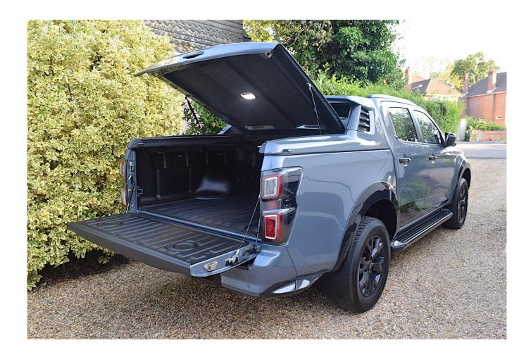
The pick-up bed area is of course smaller with a double cab than a normal pick-up, but still very roomy. Among the notable good points in this area on our test vehicle, were a tailgate damper, also the step built into the rear bumper, for easier access to the load compartment (this step is a feature of all the D-Max models).
