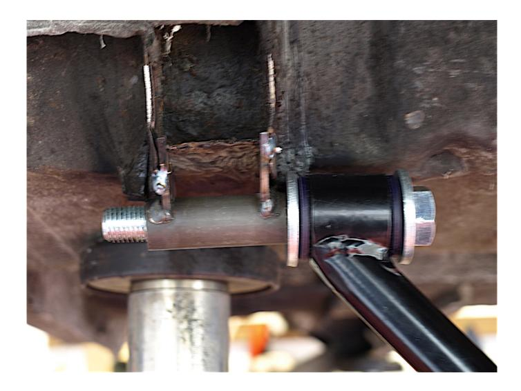
Above we can see the "A" frame used to locate each mounting piece, which are held in place by G clamps.
