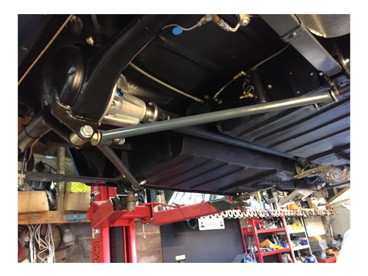
Now, referring to our first general layout/'schematic' image at the start of this feature, and the photograph below, select the correct profiles for the LEFT and RIGHT vertical brackets. They may need a little bit of adjustment to make them a good fit.
