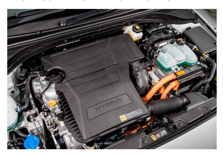
With the 1.6 GDI direct injection petrol plus 32 kw electric motor there is no compromise with the hybrid powertrain. It's smooth, has adequate power and seamlessly switches
