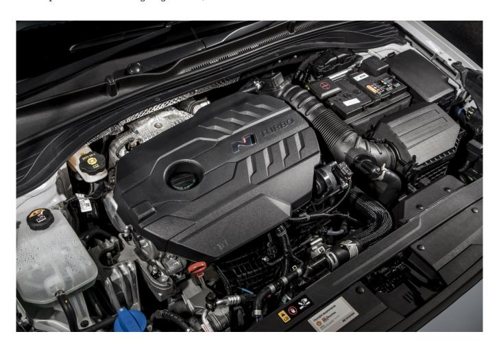
The sophisticated four-cylinder turbocharged direct injection petrol engine (T-GDI) is a good starter, pulls very strongly with 378 Nm (279 lb.ft) of torque from 1,750 rpm and yet uses its six speed gearbox to stretch its economical legs as well to almost 40 mpg.
