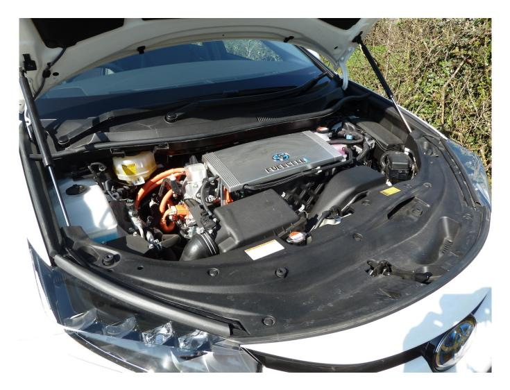
The underbonnet-mounted power control unit manages the power produced by the fuel stack and separate nickel-metal hydride battery (which stores energy recovered during decelerating and assists the fuel stack when more power is needed during acceleration), and governs power supply to the electric propulsion motor.
