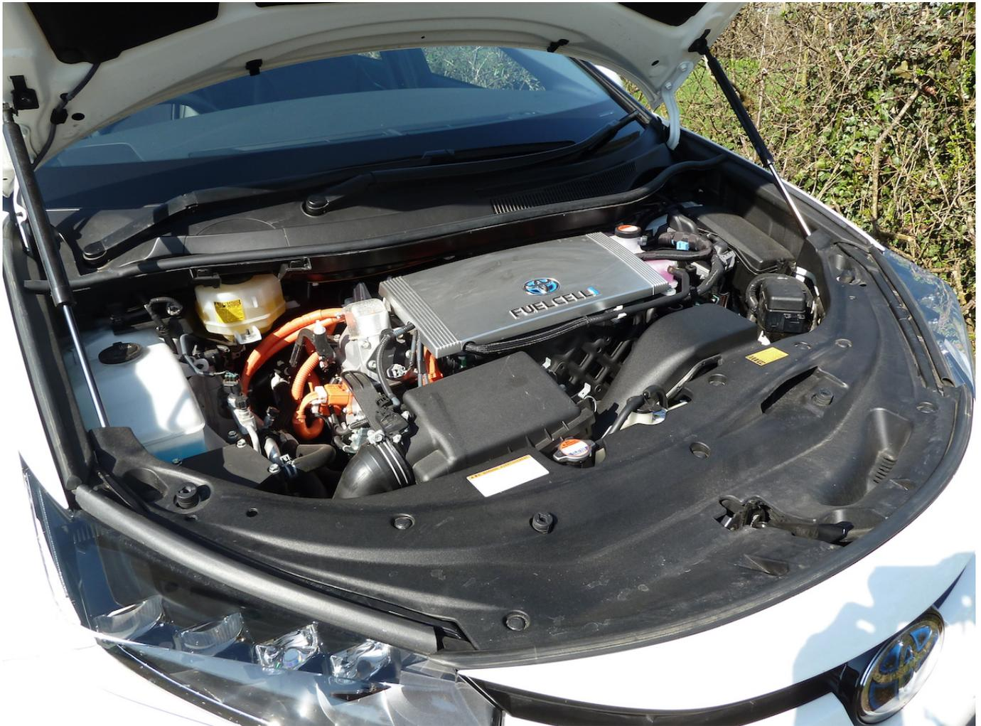
The underbonnet-mounted power control unit manages the power produced by the fuel stack and separate nickel-metal hydride battery (which stores energy recovered during decelerating and assists the fuel stack when more power is needed during acceleration), and governs power supply to the electric propulsion motor.
