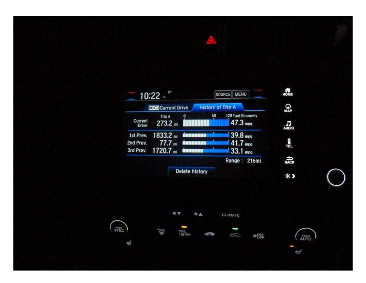
On this CR-V, Honda's on-board computer system display can be set to display previous average fuel consumption figures (obtained between re-sets of the twin 'trip meter' mileage recorders).
