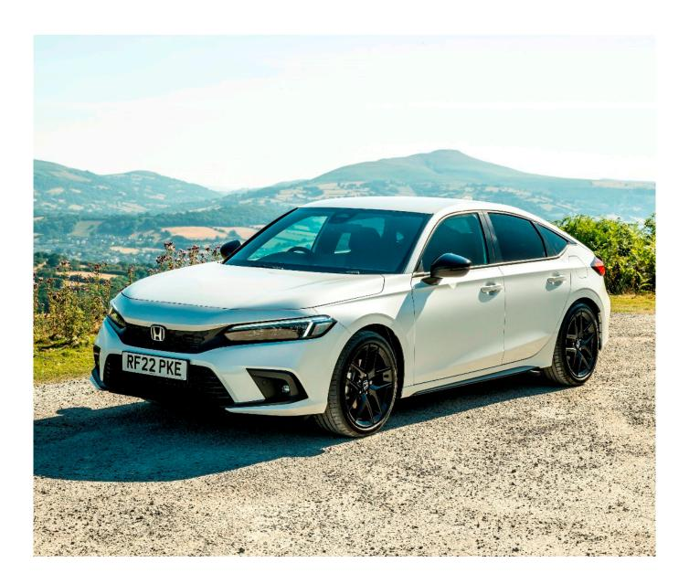
The increased size of the new Civic and the electric motor would normally add weight to the car but it's been mitigated utilising a resin tailgate and aluminium bonnet as well as a compact electric transmission that has no traditional gears, saving parts and servicing.
