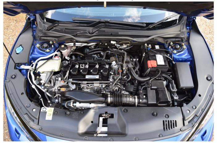
I found that the engine was eager to pull strongly from around 1,400 rpm. In fact for manual transmission variants, the maximum torque of 240 Nm or 177 lb.ft is delivered all the way from 1,900 rpm to 5,000 rpm (for the record, maximum torque in the CVT model is 220 Nm or 162 lb.ft).
