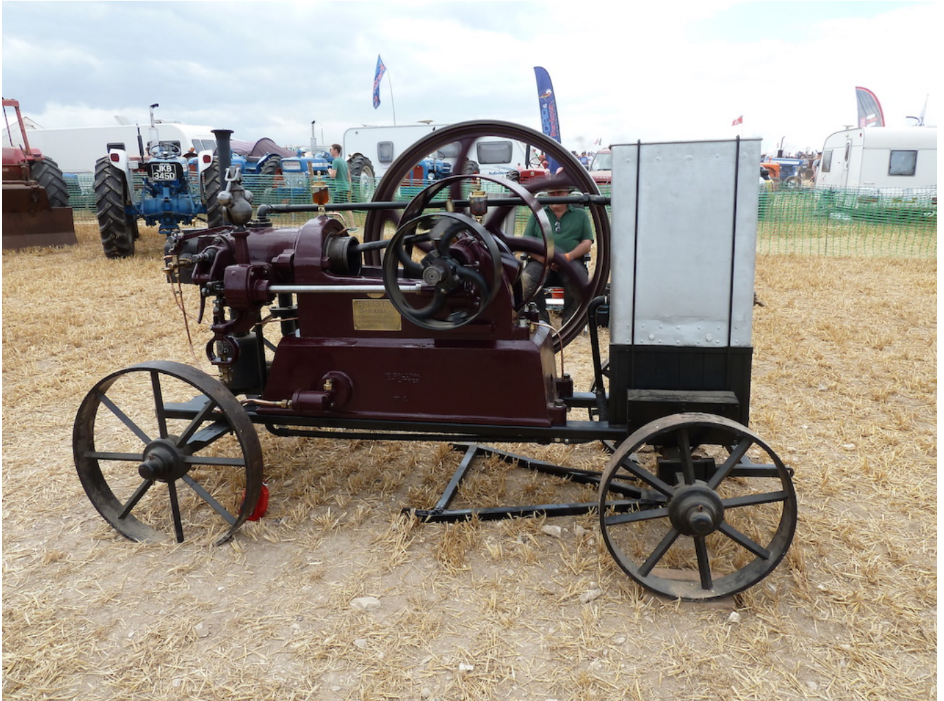
1910 5hp hot bulb R. Hornsby and Sons oil engine.
