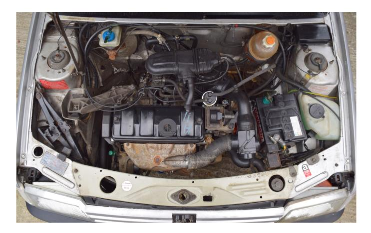
Our engine is fed by a single-barrel carburettor (so it has a choke control too); other 205 variants had a twin-barrel carburettor or fuel-injection.
