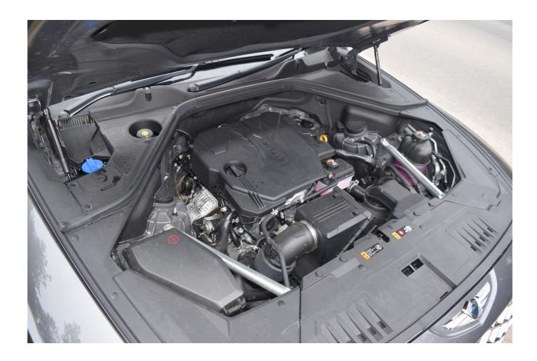
Propelling this large, all wheel drive SUV is a four cylinder 2.5 litre turbocharged petrol engine, supplied with fuel by a twin injection system and developing 304 horsepower at 5,800 rpm, plus 422 Nm (311 lb.ft) of torque, which is delivered from 1,650 to 4,000 rpm.
