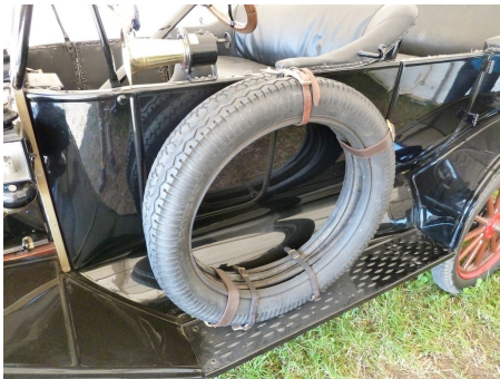
Taking no chances... twin spare tyres ('covers') on the left-hand running board.
