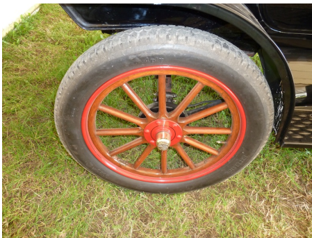
Large diameter (30 x 3 in. front, 30 x 3.5in. rear), wooden-spoked 'artillery' wheels.
