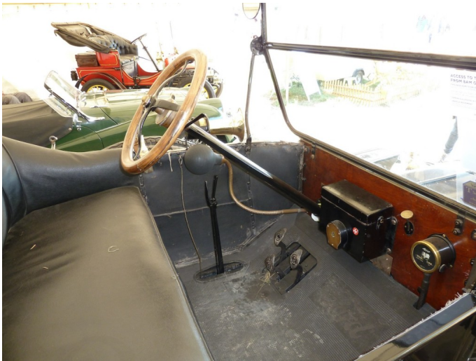
The Ford's controls; a steering wheel, two hand levers, three pedals and a floor-mounted parking brake lever (please see text).
