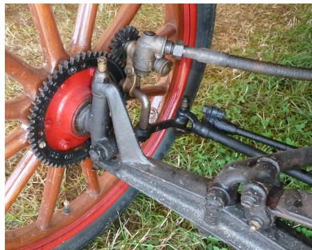
Beam type front axle; note speedometer drive (which works a treat).
