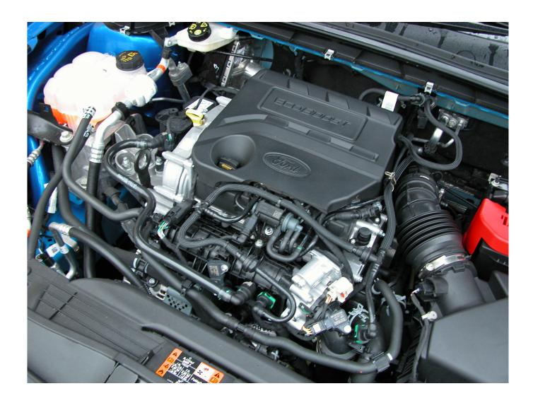
Ford's latest 1.0 litre 3-cylinder EcoBoost engine options also include a mild Hybrid model with 125 hp and also the original non-Hybrid version 125 hp unit but that offers less fuel economy and torque performance.
