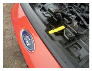
What a good idea... No need to fumble around trying to locate the engine bay's bonnet release handle on this Fiesta; it is finished in bright yellow, and very easy to find when required. Well done Ford!
