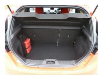
The boot is deep, wide and reasonably long from front to back; the rear seats split/fold on a two thirds:one third basis. One minus point is the high load sill, over which luggage has to be lifted.
