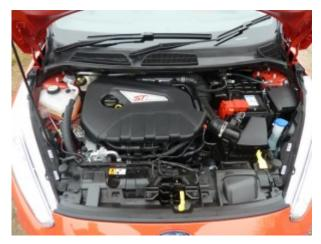
The engine bay is tightly packed; the willing 182 PS 1.6 litre turbocharged EcoBoost motor is produced at Ford's Bridgend plant.
