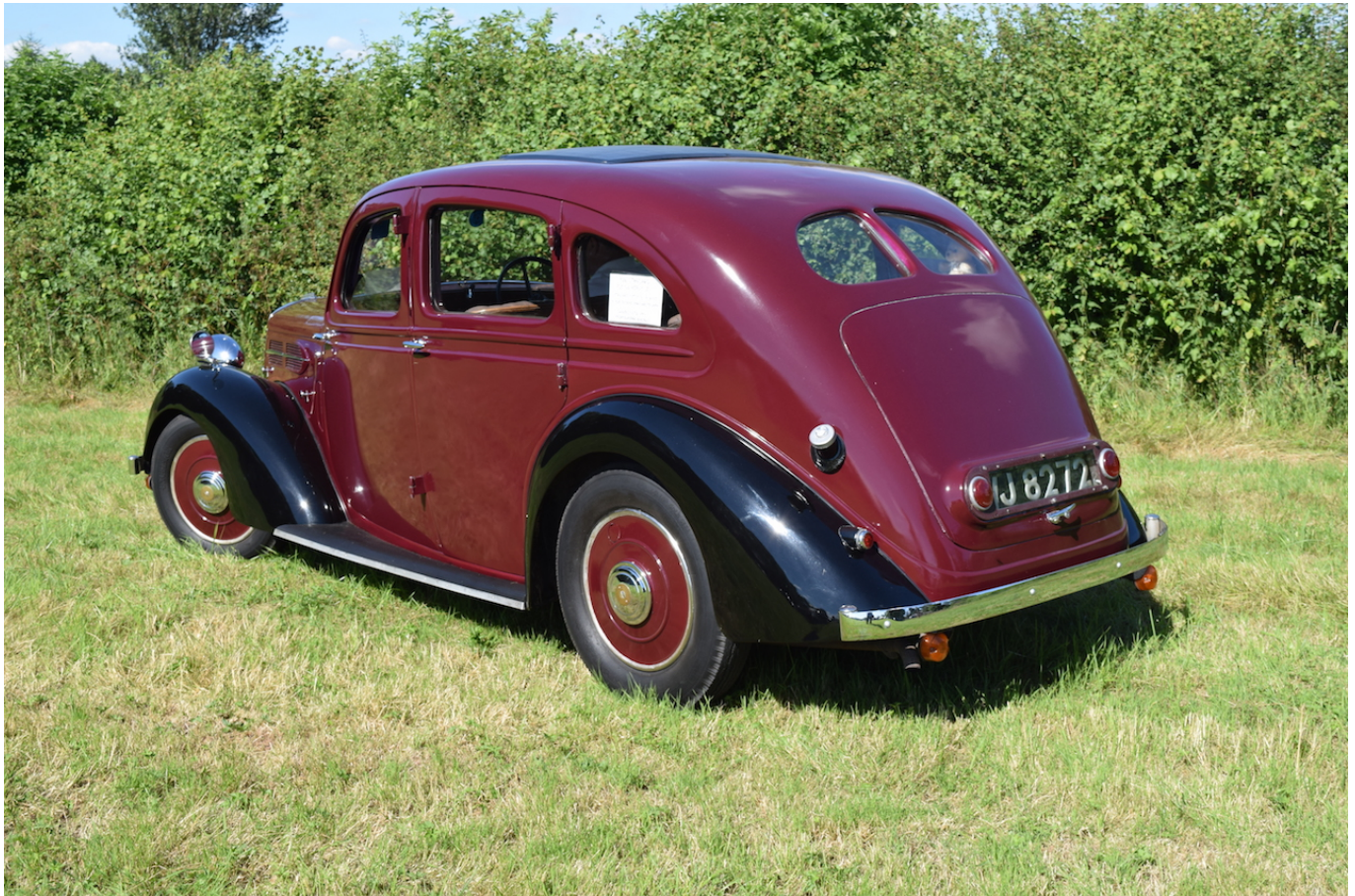
Heavy Twelve rear view shows the 'beetle back' design, luggage boot (with top-hinged lid) and rear-hinged doors, front and rear.
