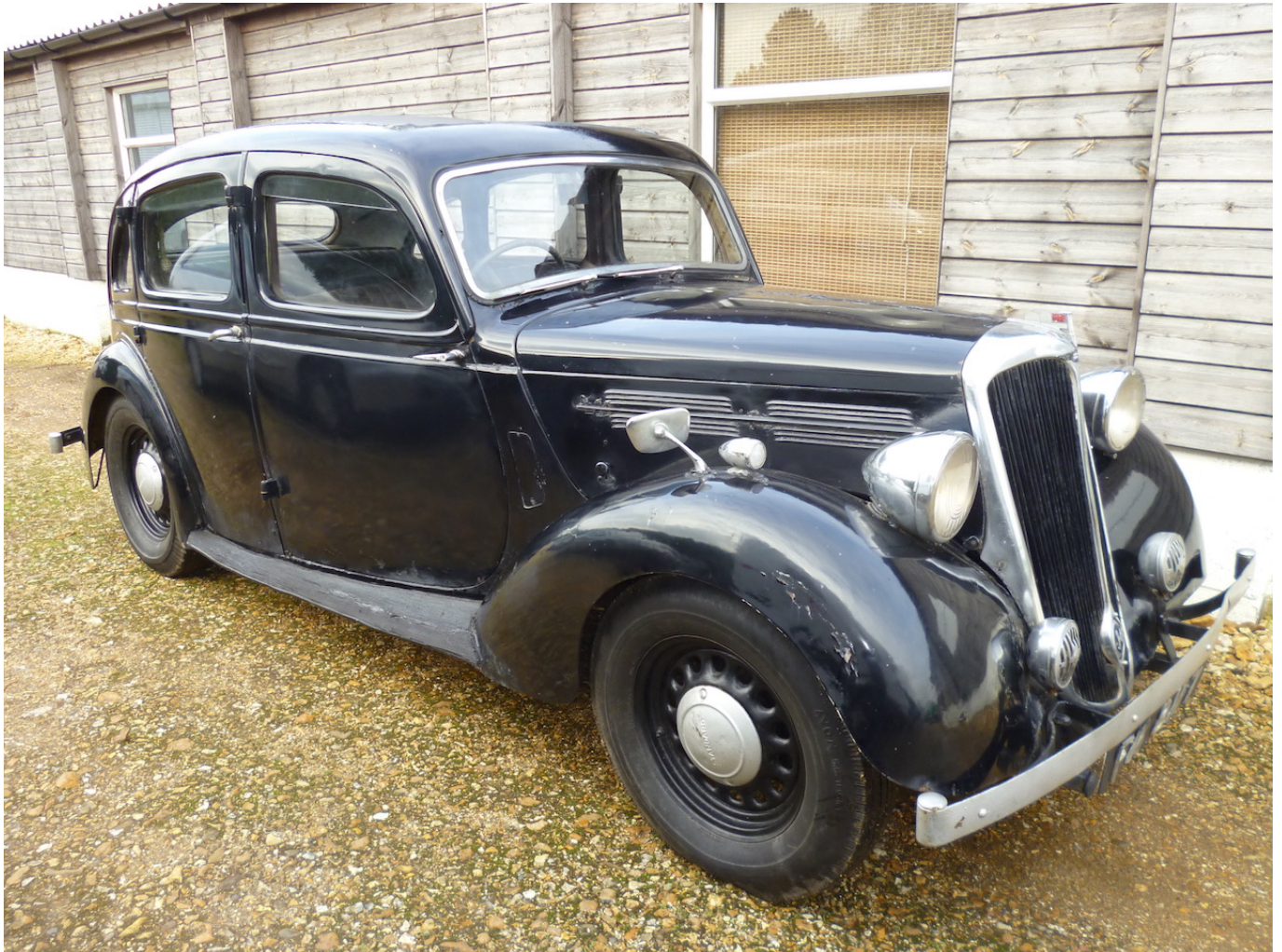
For the 1937 model year, a new Flying Fourteen arrived, looking similar to the original Heavy Twelve but with a 1776cc engine. Note the Easiclean wheels and new style of hub caps, each secured by two screws (the first use of this type by Standard).
