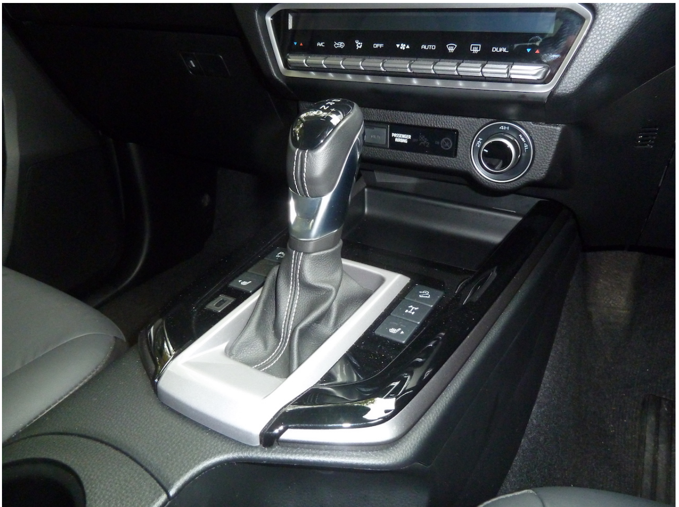
Auto transmission lever, rotary control for drive mode selection, and heating/ventilation 'buttons' all logically positioned and within easy reach of the driver.
