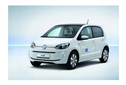
The e-up! Will be powered by an 82PS motor, which will enable the car to reach 62 mph from rest within 14 seconds, and it is said that it will have a range between charges of 150 km (about 100 miles). Its battery can be recharged to up to 80 per cent of its storage capacity with half an hour.
