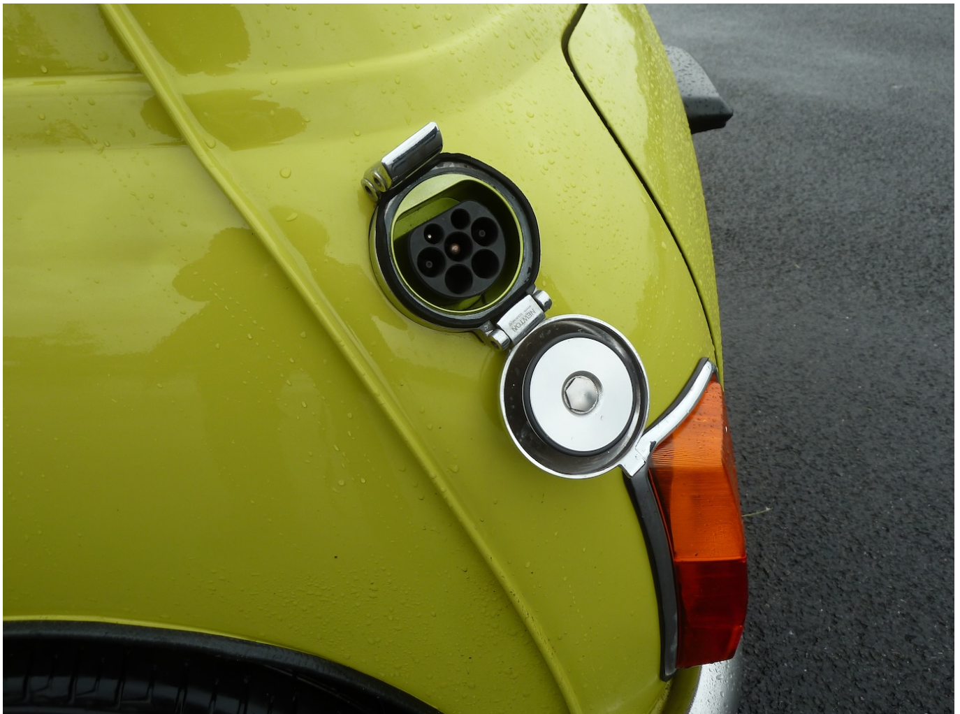
Clasic Mini converted to electrical propulsion. Photo © Kim Henson.
