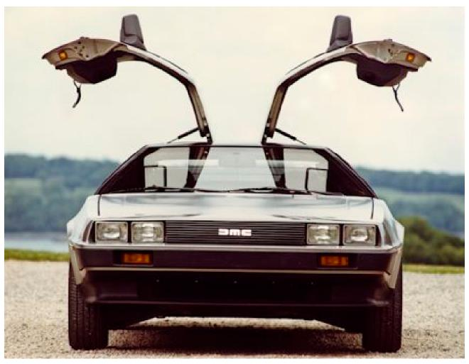
'Open wide'! A DeLorean DMC-12 showing off its gullwing doors. (Photo courtesy Virtual Motorpix).
