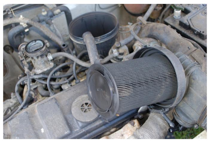
A choked air filter like this will not allow the engine to 'breathe' as designed and this will adversely affect performance and fuel consumption. Check/renew at least as often as specified by the car manufacturer. Use high quality filters too...
