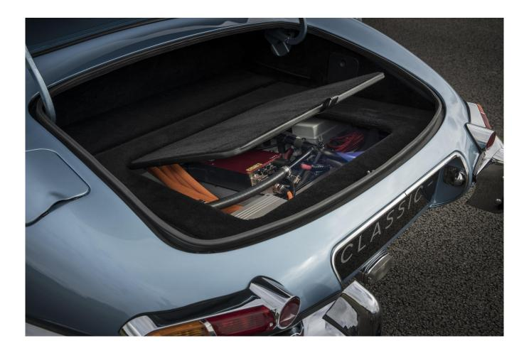
Using an electric powertrain with similar weight and dimensions to the outgoing petrol engine and transmission means the car's structure, including suspension and brakes, has not changed, simplifying the conversion and homologation. It drives, handles, rides and brakes like an original E-type. Front-rear weight distribution is unchanged.
