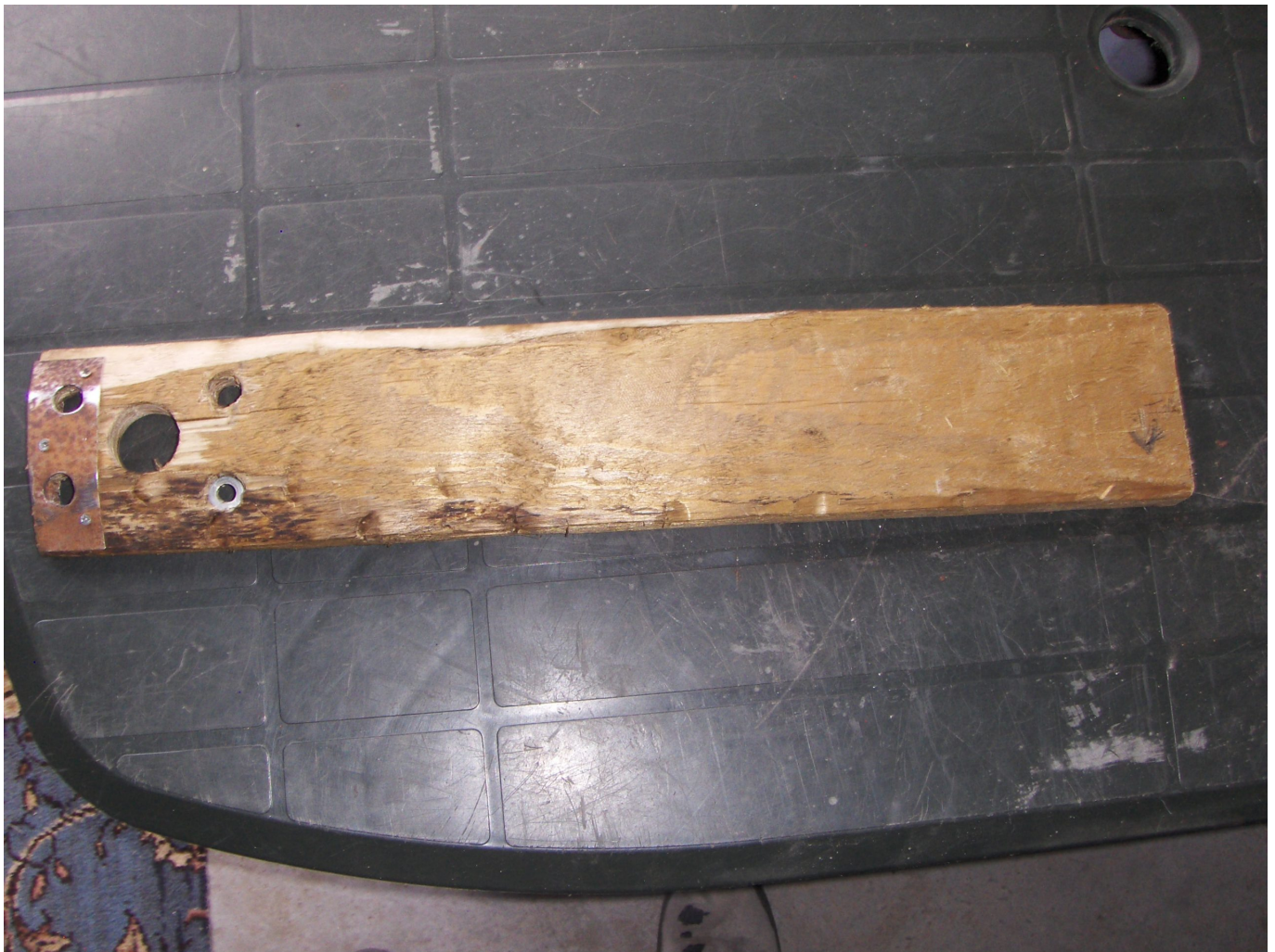
Special tool photo 2. Note: 1/16 inch Steel brace fitted at top to prevent wood crumbling.
