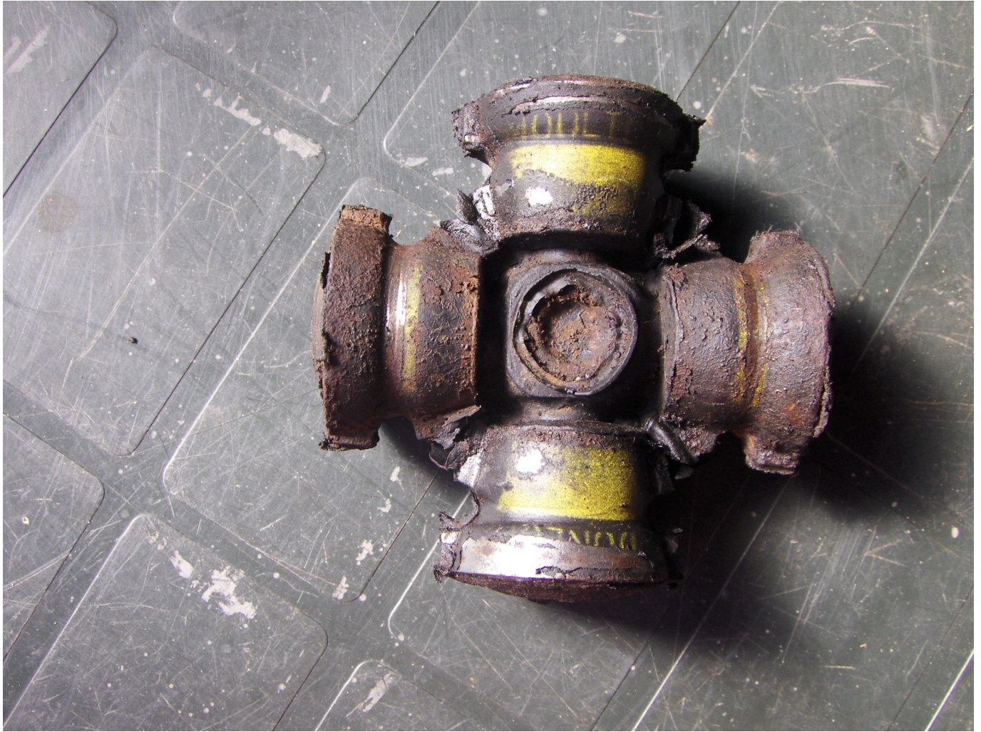
Cleaned up doughnut - early style but still in good condition. (Made by Dunlop).
