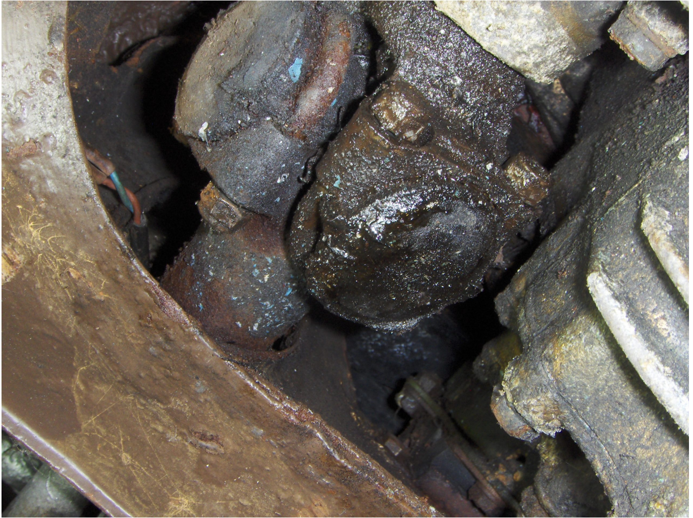
Oil bound inner UJ/doughnut connected to driving flange before dismantling.
