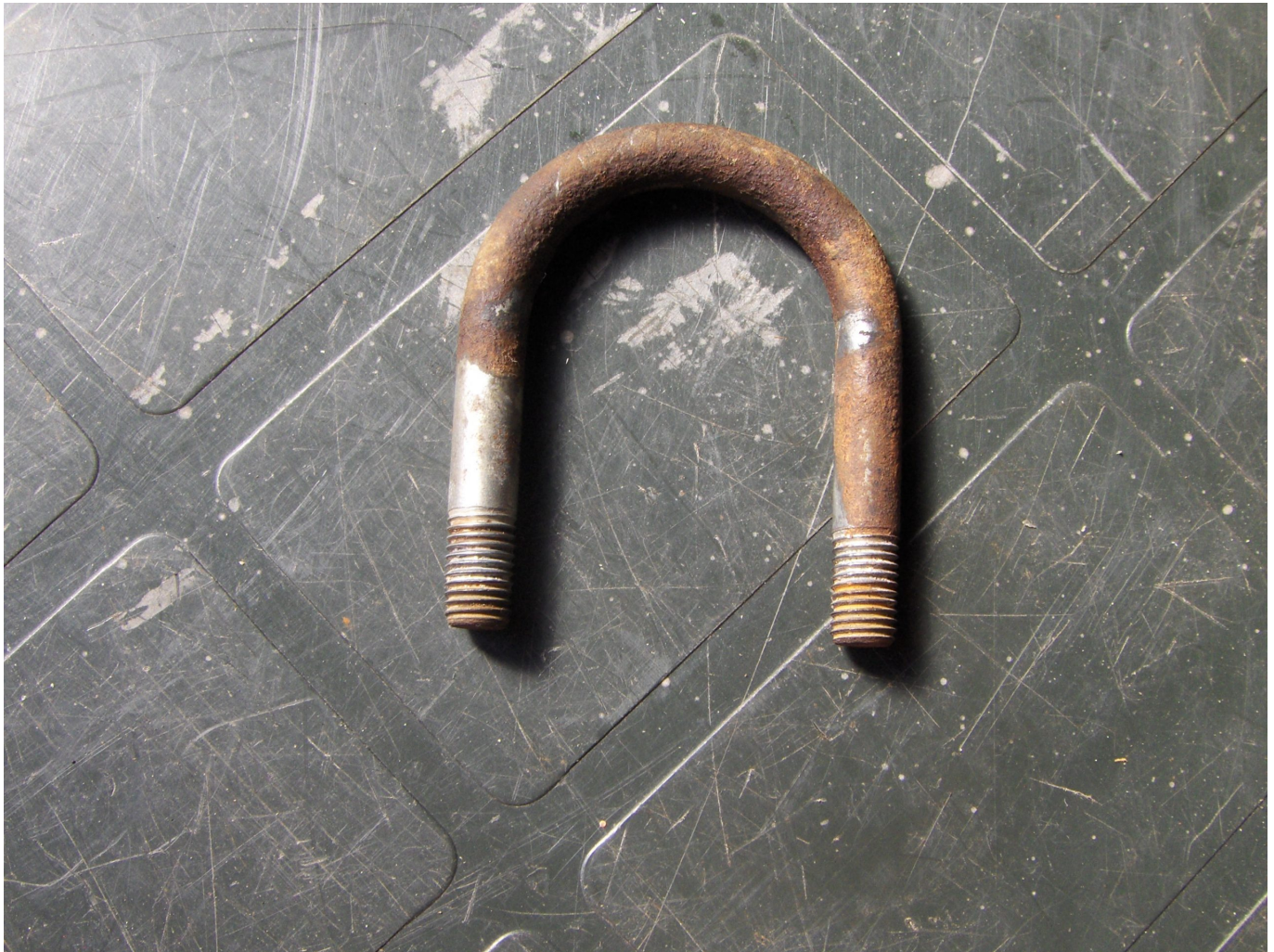
Cleaned U bolt, note shine midway along in rust on both sides indicating wear point.
