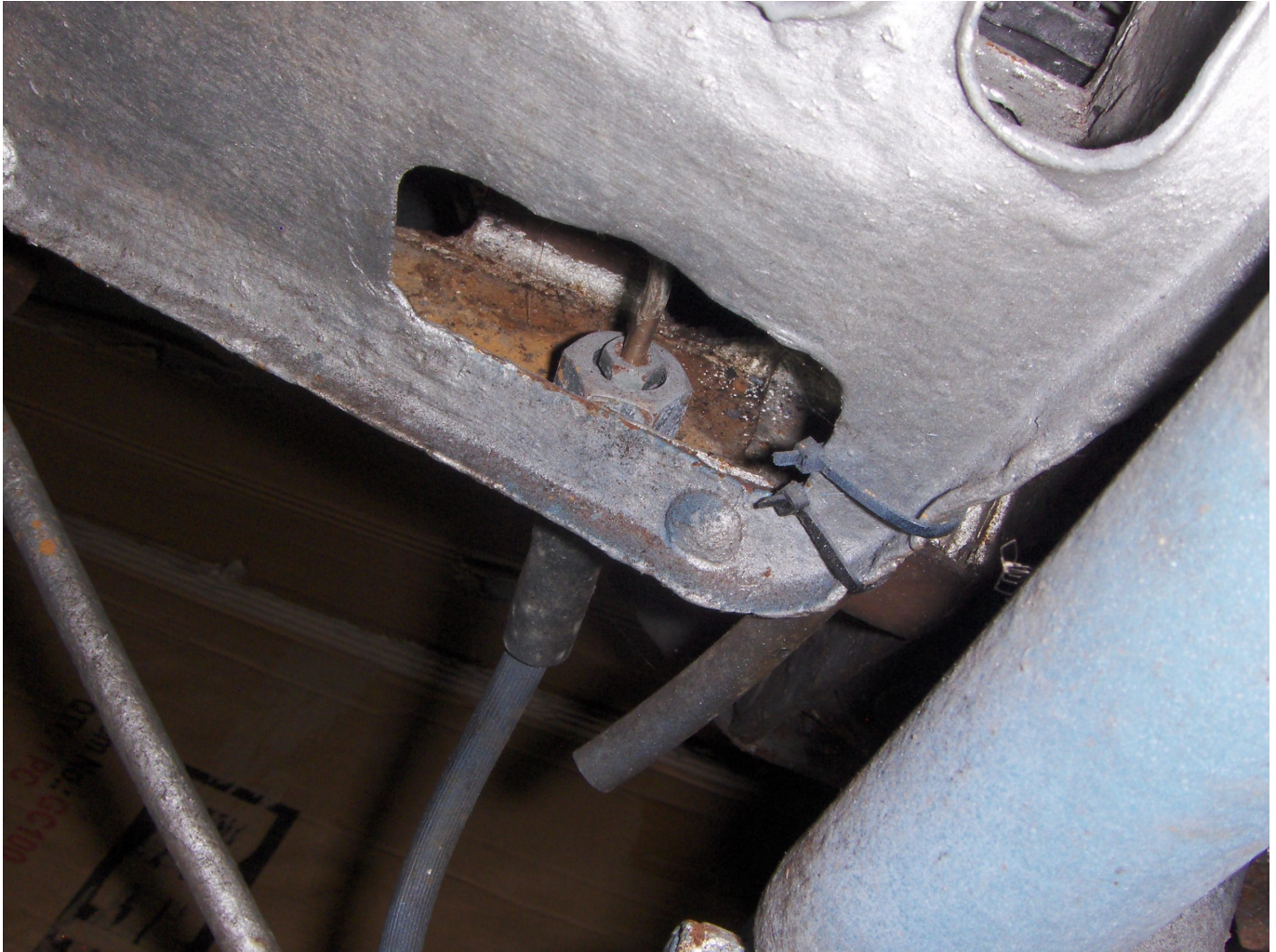
Awkward/fiddly front brake pipe connection through hole in lower inner wing.
