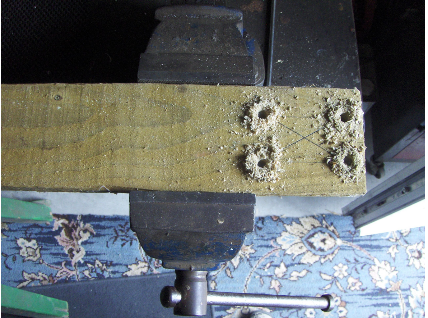
Special tool photo 1. Holes being drilled – larger hole for socket marked up in centre.
