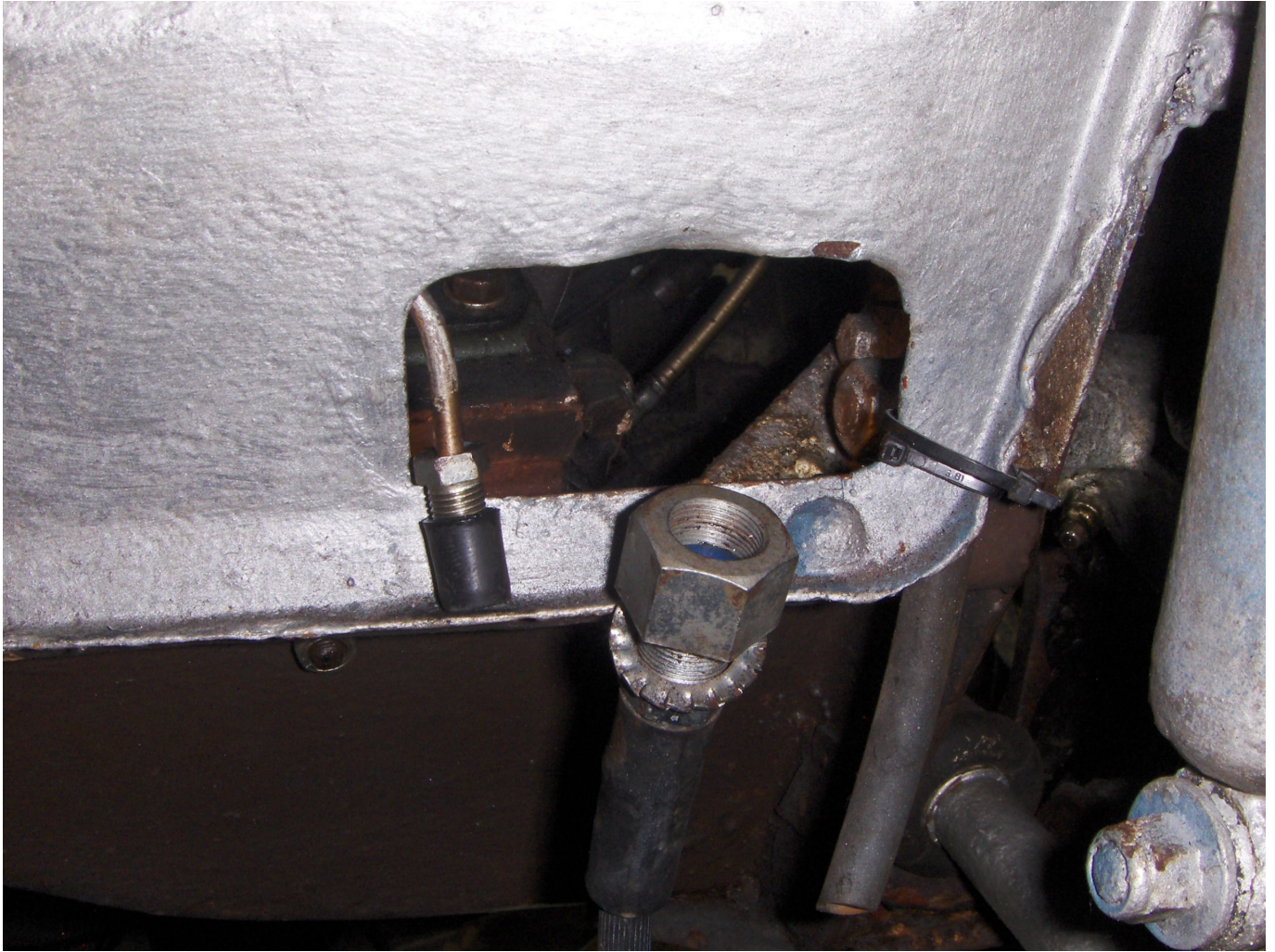
Brake pipe and hose to put together Put a plug in hose before placing in subframe hole.
