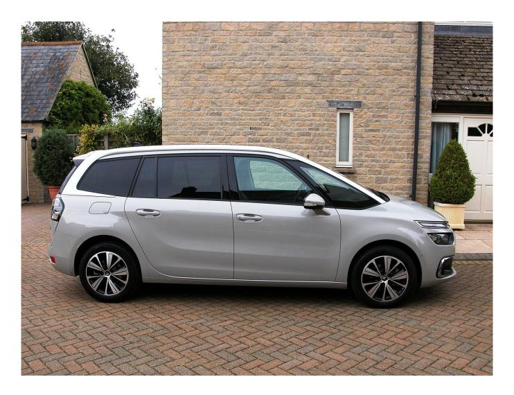
For this new road test report it's the revised 2019.5 model year Grand C4 SpaceTourer with family-friendly seven-seat accommodation we are concentrating on. Like its five-seater stablemate it has the choice of Touch Edition, Feel and Flair spec levels. The revised EU6.2 C & D Temp compliant engine line-up choices are 1.2 litre PureTech 130 petrol manual and auto versions, 1.5 litre BlueHDi 130 turbodiesel also with manual/auto gearbox options and the 2.0 litre BlueHDi 160 eight speed automatic.
