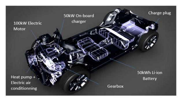
PSA image; showing electric vehicle platorm (DS3) and components.
