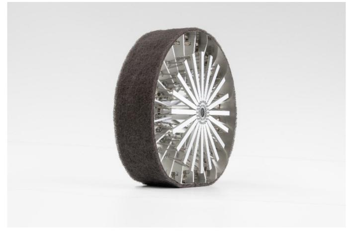
Bridgestone's expertise and knowledge of tyre contact patch will help explore the mobility challenges faced on the lunar surface, with the development of an Elastic Wheel to support the rover's weight, acceleration and braking, minimize shock absorbance, and improve manoeuvrability, enabling the rover to cruise more than 10,000 km on the lunar surface, required to accomplish the mission.
