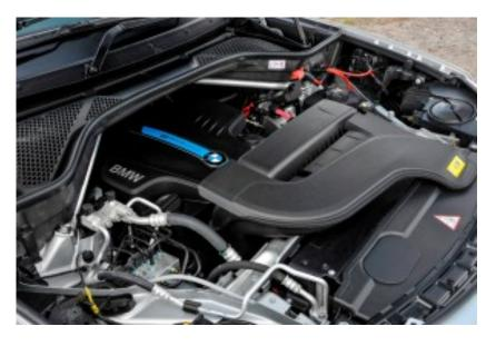
Getting to the nuts and bolts of the X5 xDrive 40e, better known as the X5 PHEV, the drive system comprises a four cylinder TwinPower turbo petrol engine and a synchronous electric motor integrated with the 8 speed Steptronic transmission. The lithium-ion high-voltage battery pack can be topped up with mains electricity from any standard domestic 240V power
