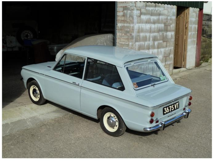
A lovely example of an early Hillman Imp, powered by a rear-mounted overhead camshaft engine. Photograph copyright Kim Henson.
