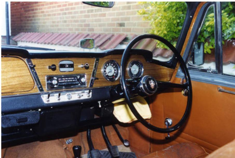
Dashboard design is simple but incorporates comprehensive instrumentation (including a temperature gauge and an oil pressure gauge).
