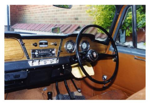
Dashboard design is simple but incorporates comprehensive instrumentation (including a temperature gauge and an oil pressure gauge).
