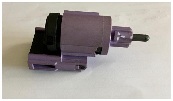
Looks innocuous, but this brake circuit controller threw out a lot of diagnostic fault codes and led to intermittent or total lack of rear brake lights. Dangerous!
