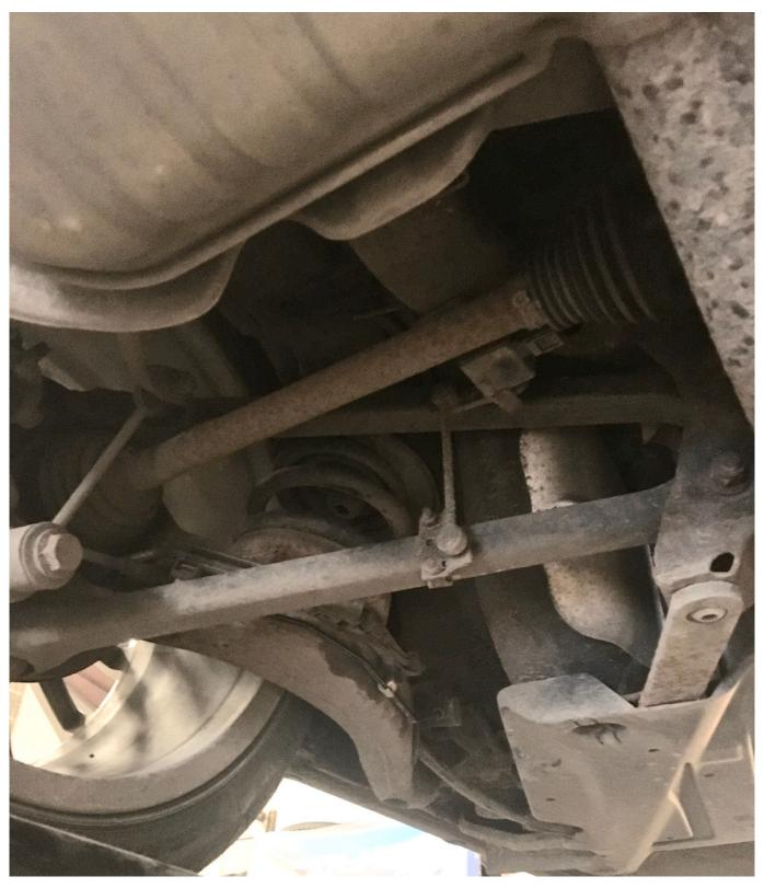
Rear brake lines replaced after evidence of scuffing, but also significant was MoT tester
