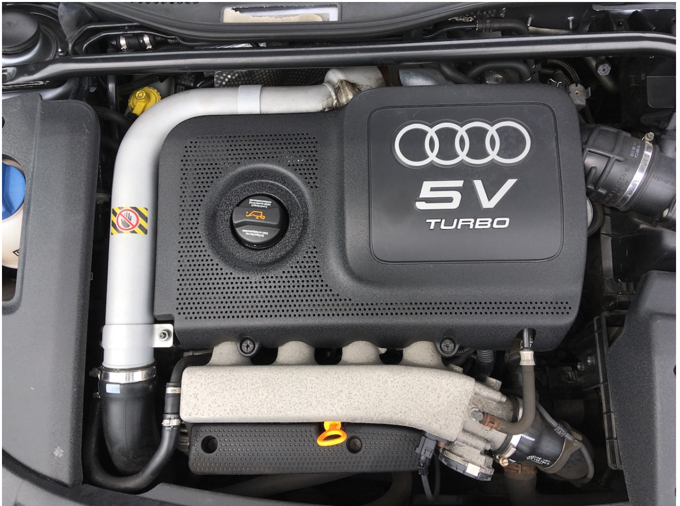
1.8 litre turbo motor with 20-valve head, modestly uprated.
