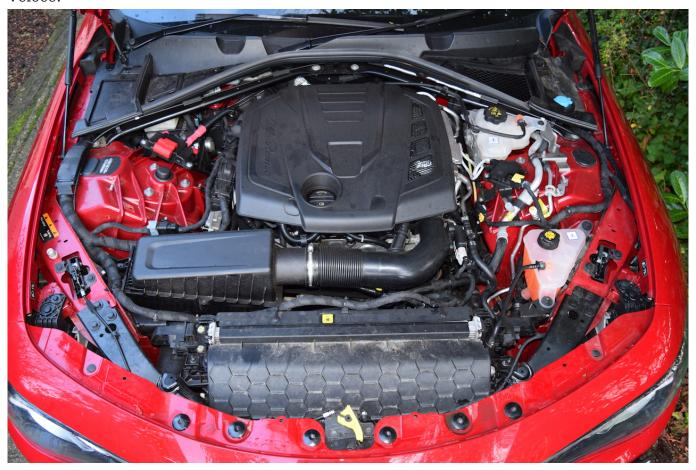
In all cases the engine is mounted longitudinally within the car, and the rear wheels are driven, via an eight speed automatic transmission.
