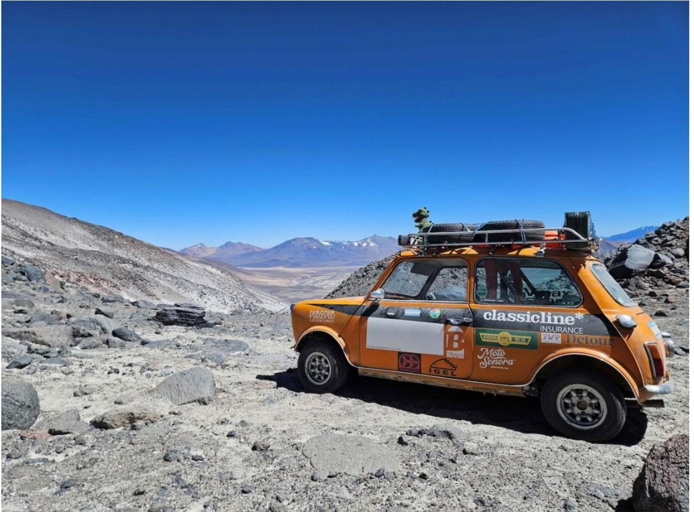
Despite daily maintenance to contend with the altitude strangling the Mini's engine of air, including regularly increasing the carburettor jet's size in line with the increasing altitude, it was a struggle to get enough fuel through to start the A-Series lump and keep it running.
