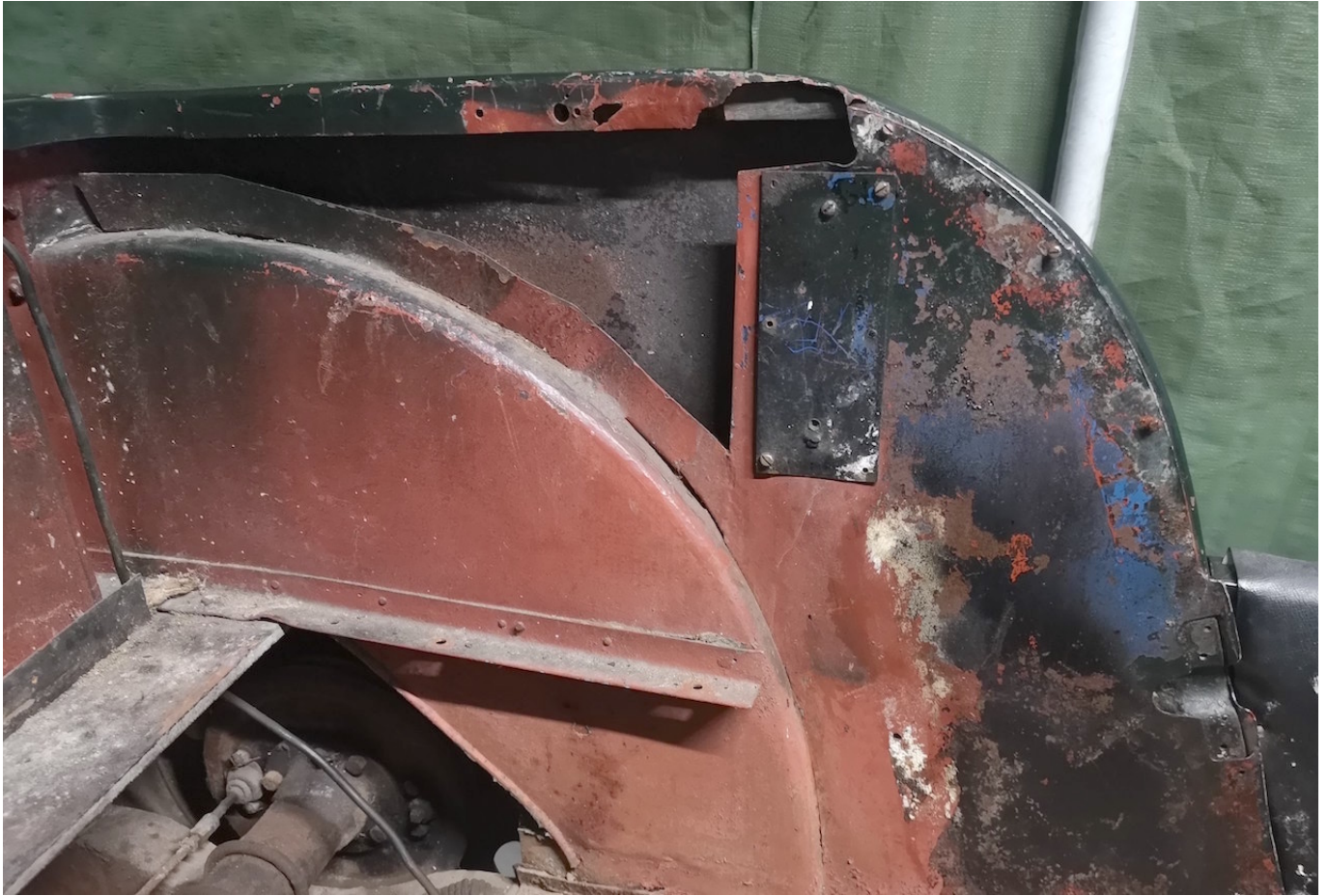
Rear inner structure - all steel!
