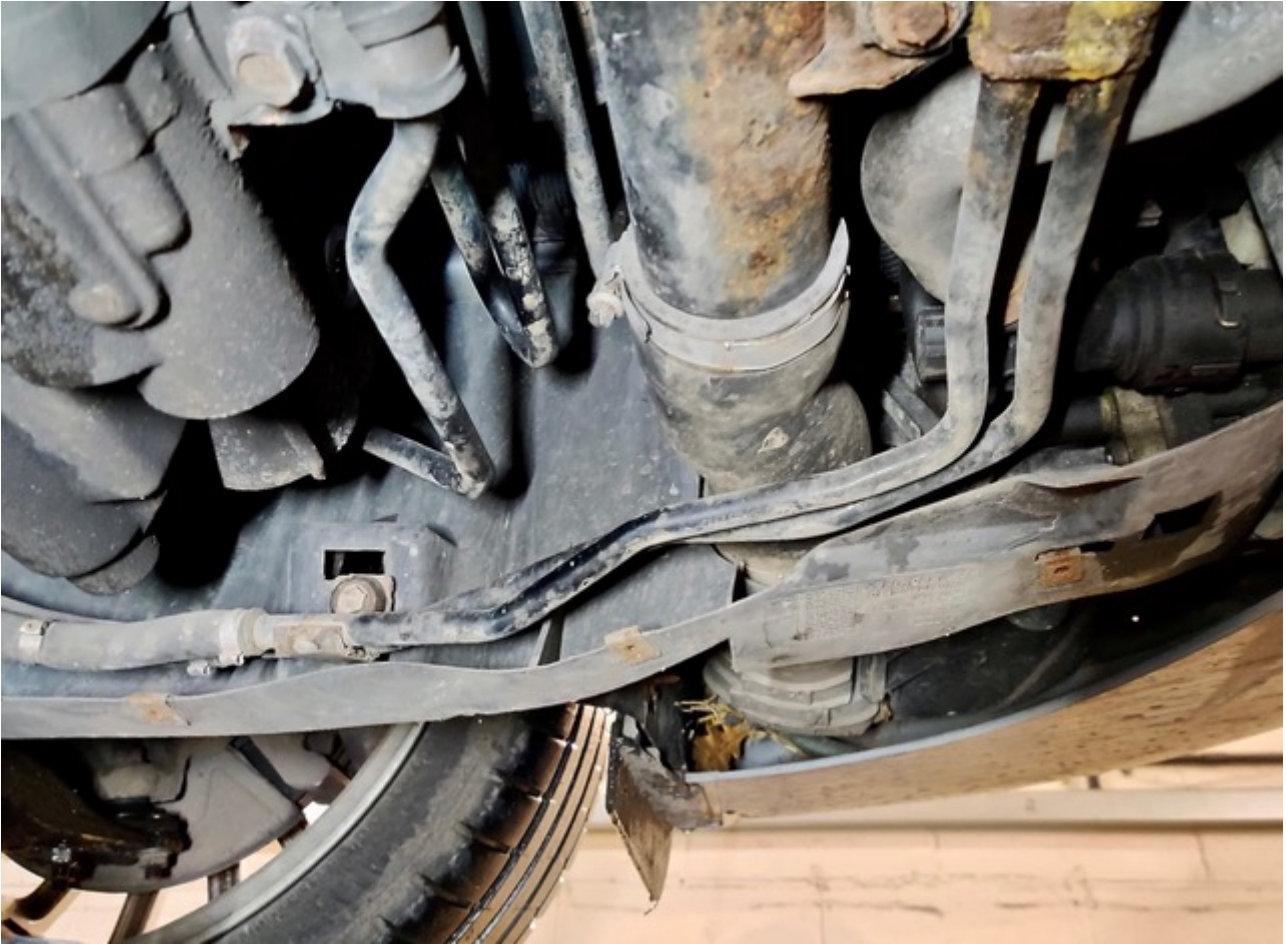
Not a pretty sight, but assorted leaks tackled, primarily from corroded power steering elongated plumbing.
