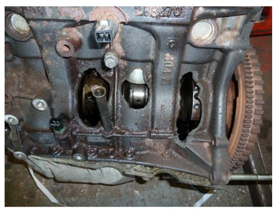
This engine was completely destroyed by a lack of oil, and in particular by the driver (we'll call him 'Silly Billy') ignoring the illumination of a warning lamp which was trying hard to advise him to stop the car and check the engine.
